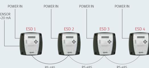
A pump set of up to 4 pumps controlled by 4 ESDs. Configuration of service pumps and back-up pumps, all regulated. Random alternation between the 4 pumps at each system start-up. Once the auxiliary pumps come into operation, all the regulated pumps operate in synchronisation at the same frequency. This operational mode enhances the effectiveness of the pump set and cuts down on the start-up and shutdown cycle for pumps.
