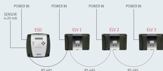
1 single ESD regulating the service pump and operating up to 3 auxiliary pumps in DOL start-up. Configuration of the master pump operating at variable speeds and 3 auxiliary pumps with in cascade operation start-up for greater flow demands. Random alternation in the start-up of the auxiliary pumps.
