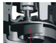
**Large chamber** between the impeller and the aspiration cone which allows suspended solid particles to pass through. Drainex 200, 45 mm. and Drainex 300, 60 mm.
