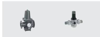
Brass and cast iron pressure reducing valves to reduce outlet pressure between 1.5 - 8 bar, maximum inlet pressure of 25 bar for brass and 16 bar for cast iron.
