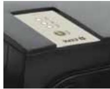
Electronic device with reset button and LEDs showing line, pump in operation and failure.
