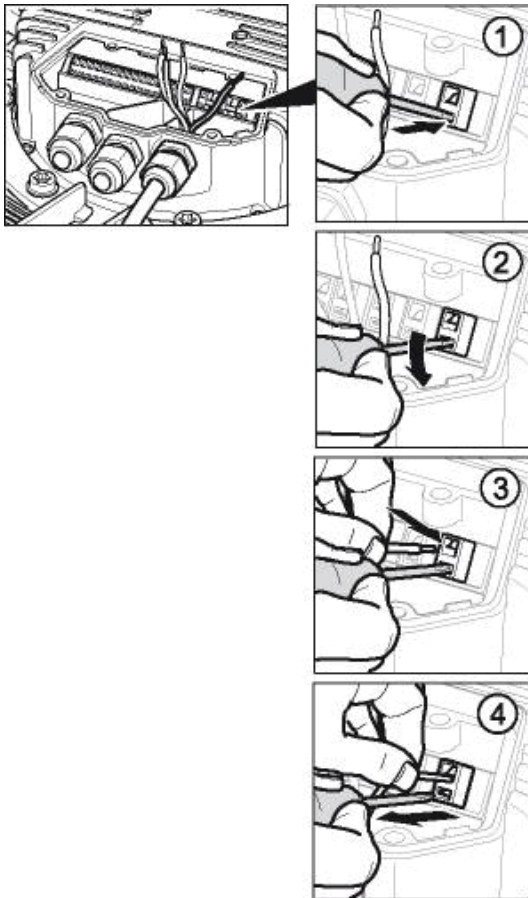
Fig. 2: Connecting wires to terminals
