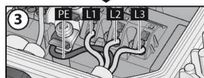
Fig. 2: Connecting wires to terminals
