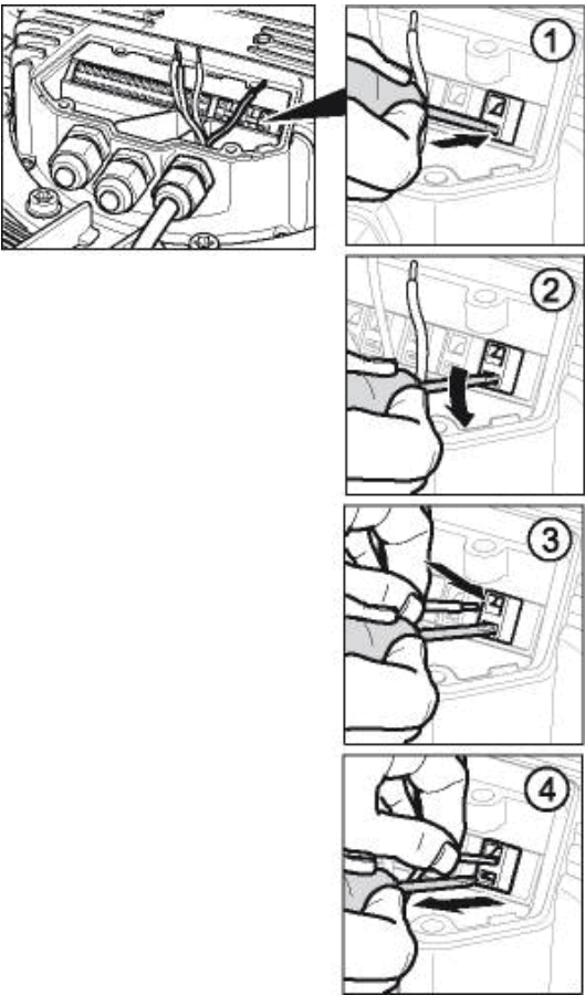
Fig. 2: Connecting wires to terminals
