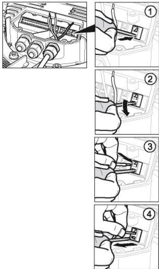
Fig. 2: Connecting wires to terminals
