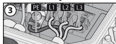
Fig. 2: Connecting wires to terminals
