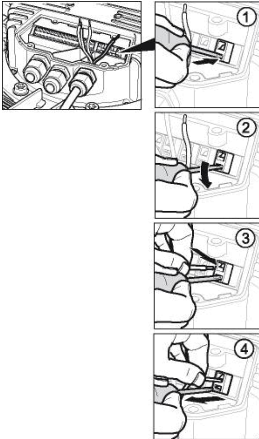
Fig. 2: Connecting wires to terminals
