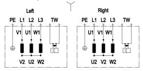
Note: Change of rotation direction by reversing two phases
