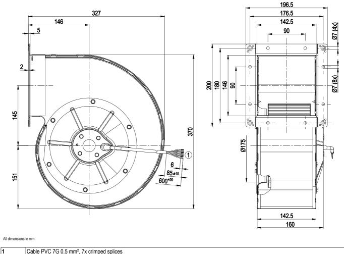
Cable PVC 7G 0.5 mm<sup>2</sup>, 7x crimped splices
