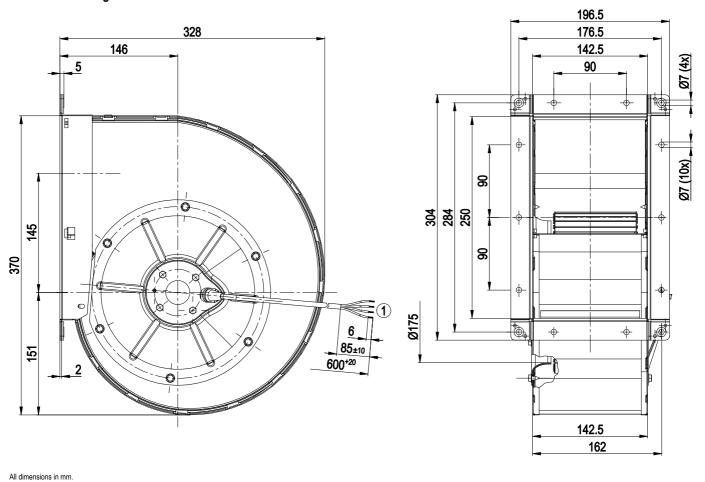
Cable silicone 4G 0.5mm², 4x crimped splices
