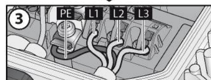
Fig. 2: Connecting wires to terminals
