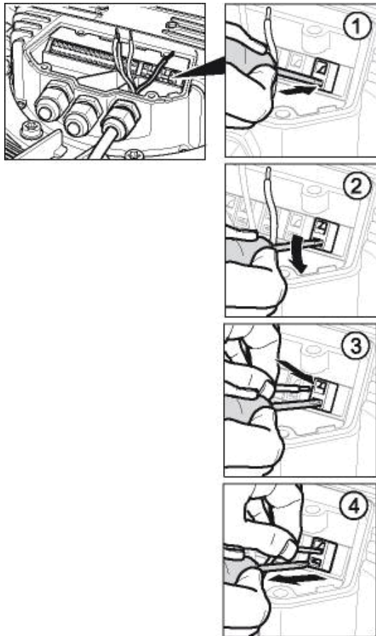
Fig. 2: Connecting wires to terminals
